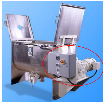
Gearmotor-driven Ross Ribbon Blender
